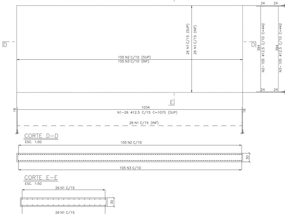
**ARMADURA DAS PLACAS PRÉ-MOLDADAS (312x)**
